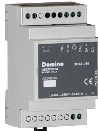
Near to the **Domino** bus terminal block, the module features a small pushbutton (PRG) for the assignment of the address and a green LED that shows the operating status; this green LED normally flashes every 2 seconds about to signal that the module is properly supplied and operating.
