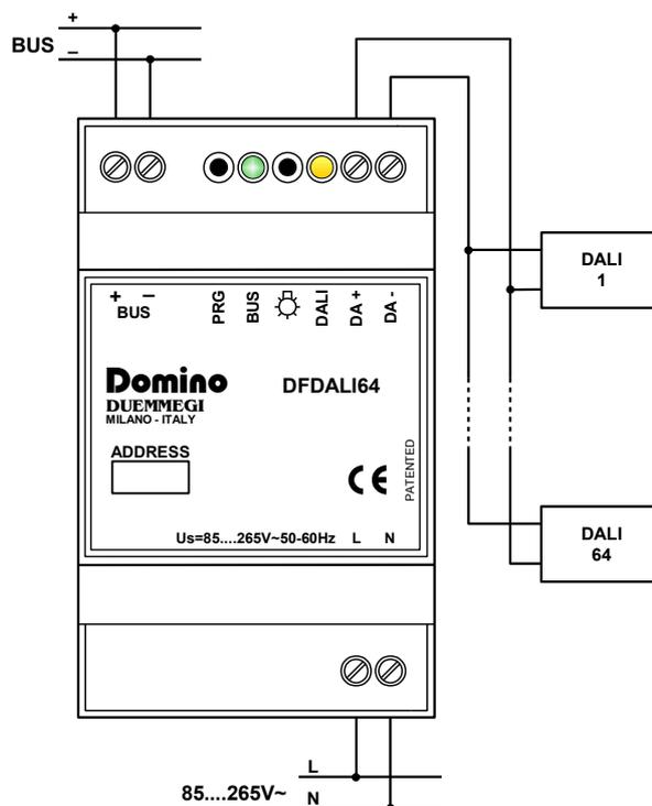
Figure 1: Connection diagram
