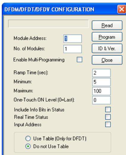
Enter in the related text box the address of DFDV module to be set; set the ramp time, the **Minimum** and **Maximum** entering the desired values in the related text boxes.
