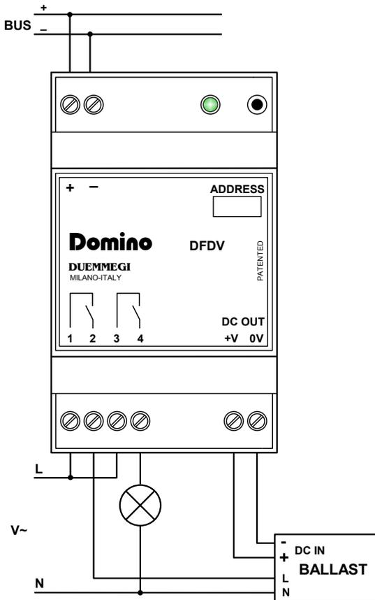
**Warning:** the output contacts of each module **CANNOT** be connected to different phases because the clearance between components do not allow this; otherwise the module may be damaged.
