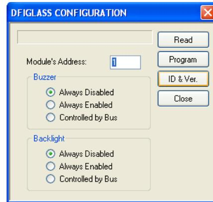
Module's Address is the address of DFIGLASS to be configured; for the backlight, like for the buzzer, 3 options are available:
