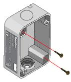
Introduce the bus through the cable bushing: pay attention to the coupling between them in order to assure the waterproof characteristic of the module. After that connect the bus cable to the 2-way removable terminal block: pay attention to the polarity.
