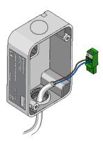
Finally, insert the removable terminal block into the related male connector.Place in the correct way the gasket on the cover and apply to the the bottom of the module: pay attention that the removable terminal block be on the opposite side of the cable bushing.
