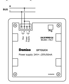
If instead DFTouch video terminal will be supplied by an auxiliary power supply, the connections to be made must be as in the following schematic diagram.
