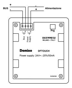
There is no polarity to be observed when using an ac power supply; anyway, if the ac voltage supplies more than one DFTouch modules, the connection +/- on the several DFTouch must be the same.
