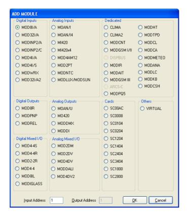
Select one of the listed modules and specify the address in the related te4 box (for mixed and some special modules, both input and output address has to be specified).
