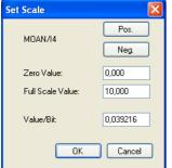
For analog modules, MCP VISIO allows the setting of the measurement scale. The figure on this right side shows 3 analog modules (MOAN/I4, MOD2PT e MODNTC) inside a group of MCP VISIO.
