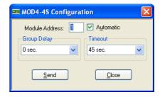
Enter the wanted parameter values and then press *Send* button. The address identify the shutter channel to be set; of course this procedure is valid if that channel was properly set for shutter operation.
