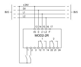
**Note:** the input section cannot be electrically insulated from the bus power supply.
