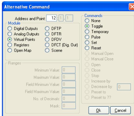
It is possible, from this window, to select a destination for the command to be executed that is different from the register 1 used for visualization. The figure shows, as example, the toggle activation of the virtual point 12. In practice, the images and text related to register 1 will be visualized, but, when clicking on that icon, a commands to virtual point 12 will be sent.
