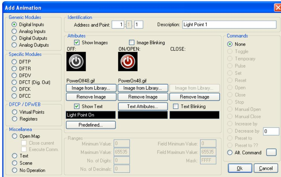
The button **OK** closes the window **Add Animation** and the created icon will be shown on the map in the top left side. The icon can be moved to the wanted position holding down **CTRL** button and the left mouse button and moving the mouse; when the position is reached, release the mouse and the **CTRL** buttons (or use the arrows buttons as described at paragraph 3.2).
