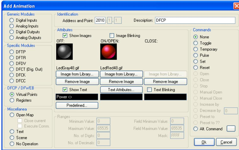
A virtual point shown on the map can be of course be controlled enabling one of the commands on the right side of the configuration window of animation.
