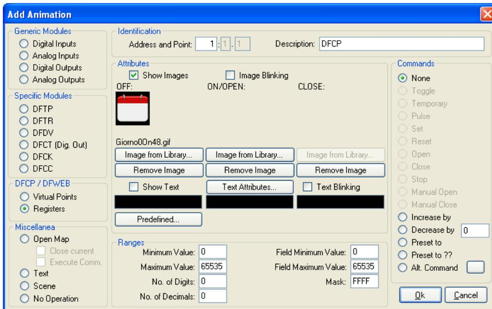
For registers are also allowed all the options related to the analog outputs (setting of Zero Value and Full Scale Value, No. of Decimals, Mask, commands Increase by, Decrease by, etc.)
