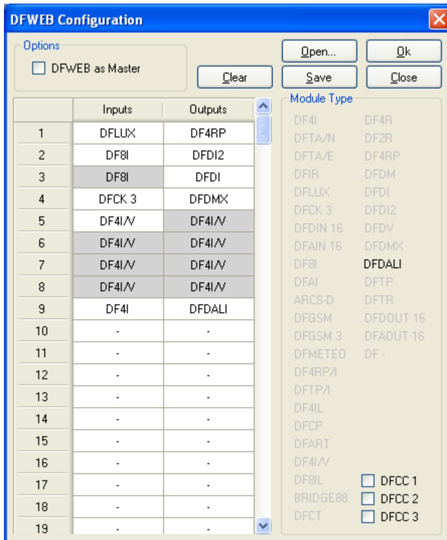
The grey boxes corresponds to the addresses automatically reserved to the modules with multiple address (in the previous example the DF8I and DF4I/V modules). Once completed, the configuration has to be saved pressing the Save button. In this way, the file **DfWebCfg.xml** will be saved (the name MUST NOT be changed); this file MUST BE NECESSARILY saved inside the XML folder of the project structure. The following figure shows the structure of a project named MyPlant.
