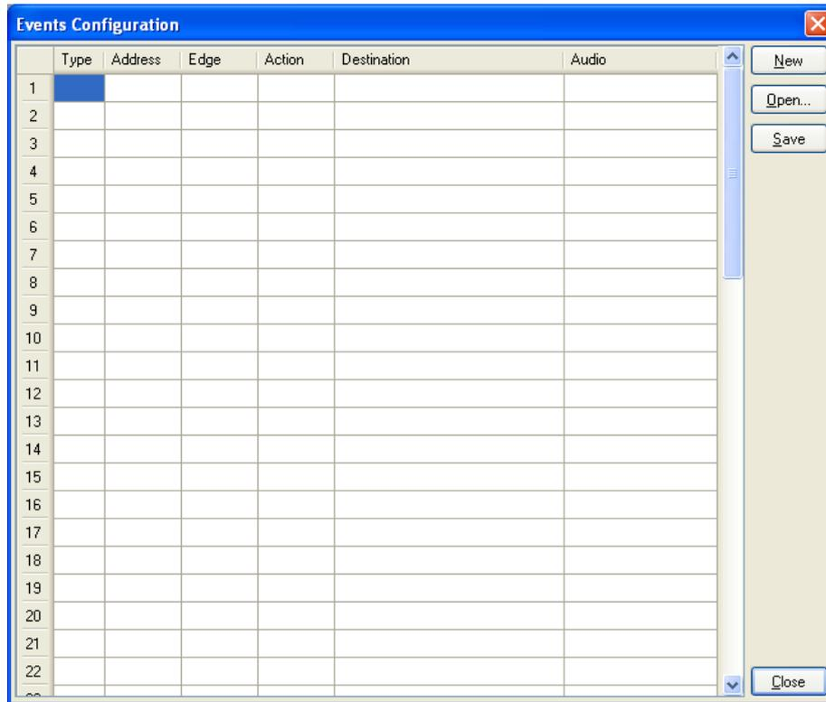
By double clicking of the left button of the mouse on any cell of the table, the configuration panel will be opened for that event:
