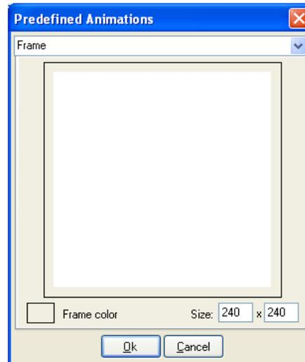
The border color of the frame can be modified selecting the option Frame Color. To change the dimension of the frame use the combination CTRL + left button of the mouse on the bottom right corner, of course after having added the frame to the map. It is possible to modify the dimension of BarGraph during the adding phase by the modify of the Dimensions field value.
