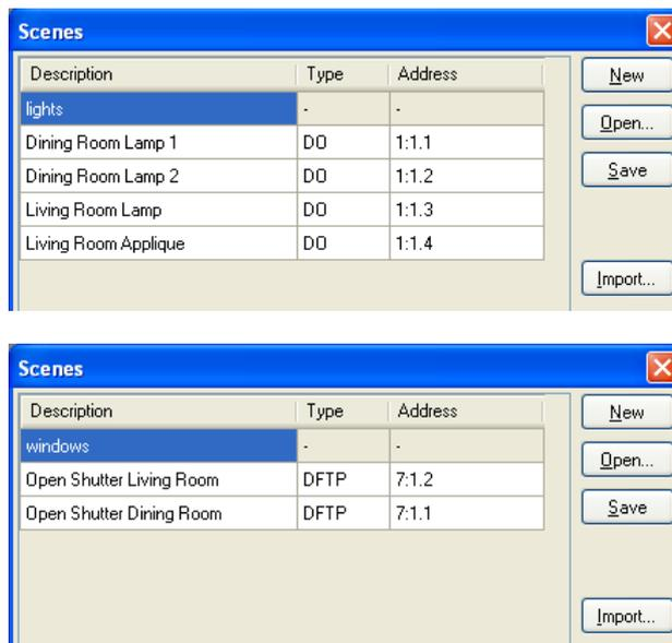
After having saved the two sceneries in the correct user folder (for example **user**), the .bin file to be transferred to WEBS module can be created.
