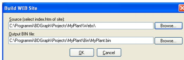
The building of the Web site consists in the creation of a .bin file containing all the involved HTML pages; this file is in a proper format to be uploaded to WEBS module and it must be saved (for instance as MyPlant.bin) inside the folder **MyPlant\Maps\Bin**. The source to be selected will be the file index.htm of the project (that must be found inside the folder MyPlant\Webs).
