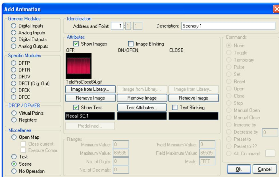
As shown in the previous window, the option Scene has been used. It is required, as unique condition for the correct operation, the insertion of the scenery number previously set inside the Address and Point text box (the scenery in the example is the number 1).
