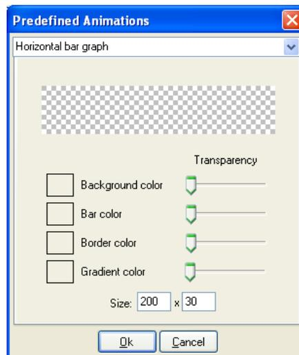
From the R.8.2.1 of BDGraph and the R.2.6 of the WEBS firmware, it is possible to set the transparency of the background of the bar, of border and of the gradient. In this way it is possible to personalize the BarGraph at each type of background and utilize.
