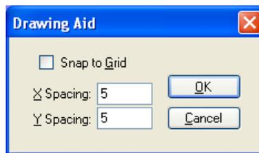
It is possible, through this window, to configure the snap X and Y value and to block the animation to the grid. In this way the positioning of various icons will be simplified and more precise. The snap value is referred to the number of pixels. On status bar will compare the information related to the lock/unlock of the grid and the information of used snap.
