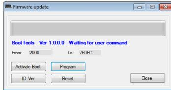
The updating of **DFWEB** main controller does not need any address, therefore click on the button "**Activate Boot**" and then "**Program**" to start updating; at the end, the program will wait for the reinitialization of **DFWEB** (10 seconds about), then the new firmware version and the IP address of the module will be shown.
