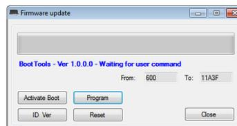
The updating of **DFTOUCH** module does not need any address, therefore click on the button **“Activate Boot”** and then **“Program”** to start updating; at the end, the program will automatically reset the module.
