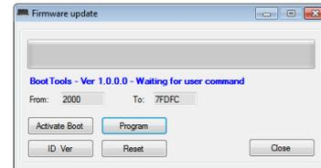
The updating of **WEBS** module does not need any address, therefore click on the button "**Activate Boot**" and then "**Program**" to start updating; at the end, the program will wait for the reinitialization of **WEBS** (10 seconds about), then the new firmware version and the IP address of the module will be shown. The button "**ID Ver**" allows to check the ID code and the firmware version; the button "**Reset**" allow resetting the module (if needed).
