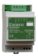
Even if the standard specifies a maximum of 32 devices for the DMX line, as a good rule do not override a total amount of 16-20 devices. If the number of devices is higher than 20, use proper line splitters to connect the devices overriding this limit.
